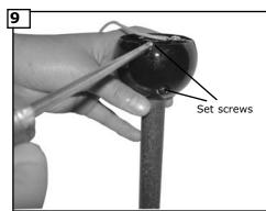
Loosen two set screws holding half ball, slide down ball and remove pin. Remove the ball.
